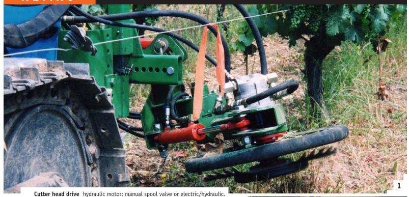
Automatic spring return cut head rolls around vines, trunks, posts, etc.
